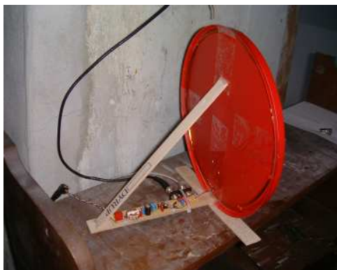
Figure 6. $20 homebrew loop antenna
