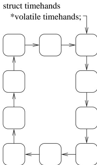
This scheme has an inherent risk that a process may be de-scheduled for so long time that it will not manage to complete the timestamping process before the entire ring of timehands have been recycled. This case is covered by each timehand having a private generation number which is temporarily set to zero during the periodic processing, to mark inconsistent data, and incremented to one more than the previous value when the update has finished and the timehands is again consistent.
