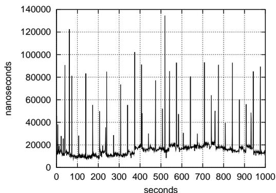
It is painfully obvious that the interrupt latency is the dominant noise factor in PPS timestamping in the second case. The asymmetric distribution of the noise in the second plot also more or less entirely invalidates the design assumption in the NTP PLL/FLL kernel code that timestamps are dominated by gaussian noise with few spikes.
