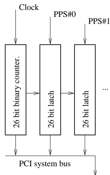
Using this setup, a standard 133 MHz Pentium based PC is able to timestamp the PPS output of
